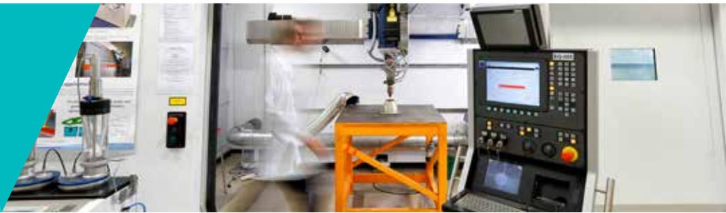
Amaero, through MCAM, has access to the southern hemisphere's only Concept Laser XLine powder bed selective laser melting (SLM) machine – the largest of its type in the world. Components up to 630mm x 400mm x 500mm deep can be produced by selectively melting fine metallic powder, layer upon layer, using a high-powered laser scanned across each layer driven directly from a computer-aided design (CAD).
