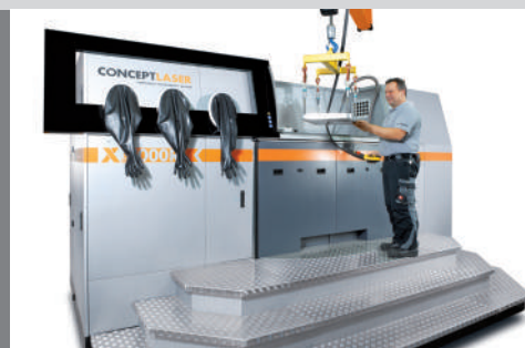
Backside of X line 2000R with crane loading during the set-up phase.
